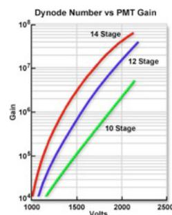
Fig. 5 gain of a photomultiplier tube
