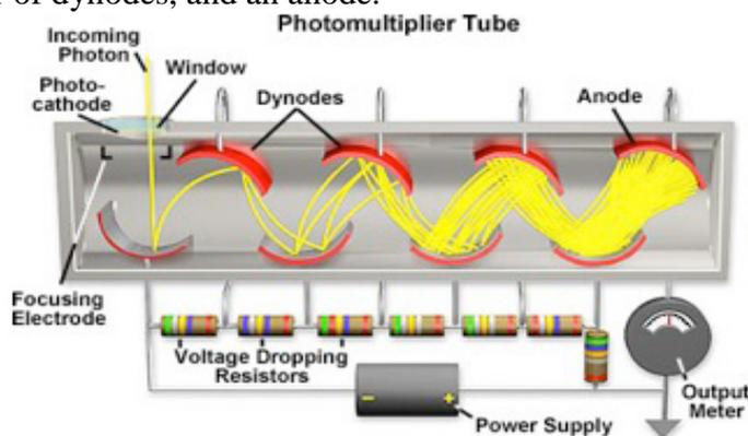
Fig. 3 Principle of a photomultiplier
